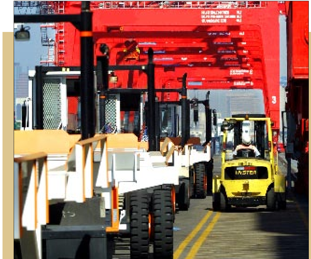
Yard hostlers line up along red gantry cranes to pick up cargo containers being offloaded from a vessel at Pier T terminal.
