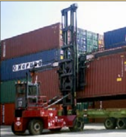
A side-loader lifts a container. These types of vehicles are being targeted by the Port's diesel emission reduction program.
