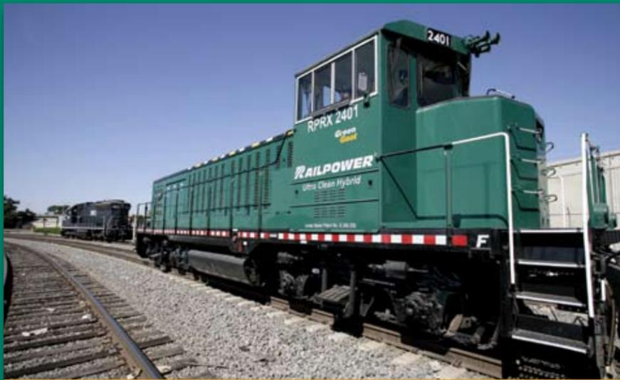
A "Green Goat" hybrid diesel-battery locomotive will be among the new, environmentally friendly locomotives to replace Pacific Harbor Line's aging locomotive fleet.
